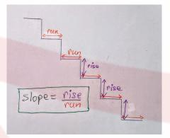
The slope, or steepness of the staircase, can be defined as,
